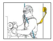
Allows the rope to be kept at a distance to protect it during certain work phases.
